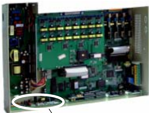
The Installation Site of D1SLCB
