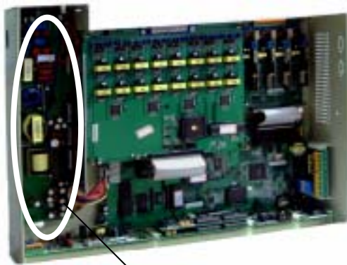
The Installation Site of D2PWUA
